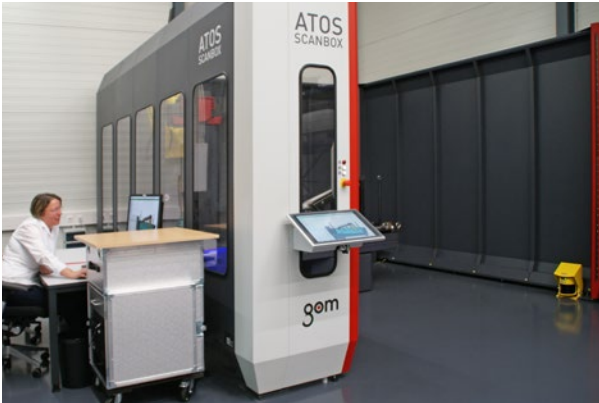
Fig. 4: Allgaier Automotive is using the ATOS ScanBox 6130, which can even accommodate and measure large car body parts, thanks to its wide entryway.
