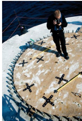
Abb. 12: Measurement with TRITOP CMM photogrammetric camera
