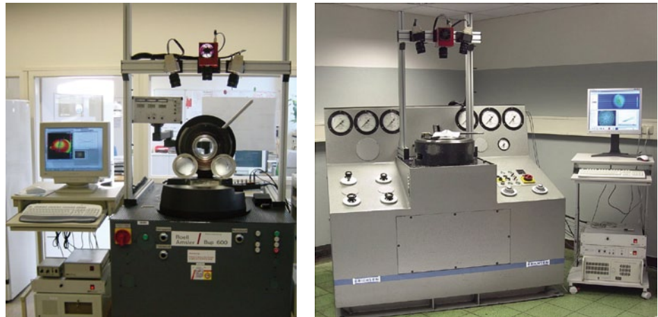
Fig. 5: Measuring setups above different sheet metal forming test machines to determine Forming Limit Curves
