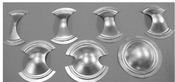
Fig. 2: Different specimen geometries, from the entire blank to strongly waisted blanks
