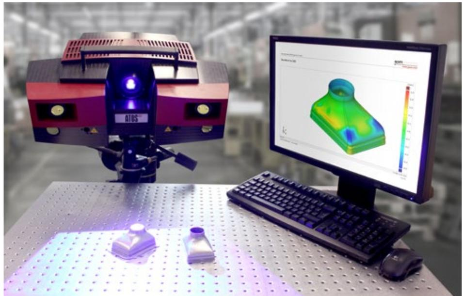
Fig. 2: Measurement and full-field comparison with CAD data using the ATOS Triple Scan 3D optical measuring system.
