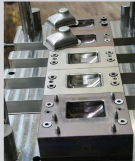
Simulation and measurement reduce the number of correction loops required for the deep drawing tool.
