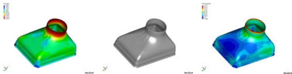
Fig. 3: The component in the Stampack simulation system during thickness distribution simulation (left). The component in the Stampack system after completing the simulation (middle). Degree of utilization of the forming limit (right).
