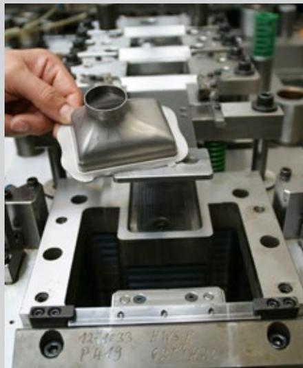
Top part of progressive deep drawing tool with untrimmed component.
