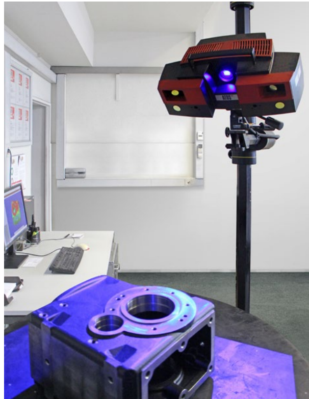
Fig. 6: The projection unit of the ATOS Triple Scan system is based on Blue Light Technology. Since the sensor works with narrow-band blue light, interfering ambient light can be filtered during image acquisition.
