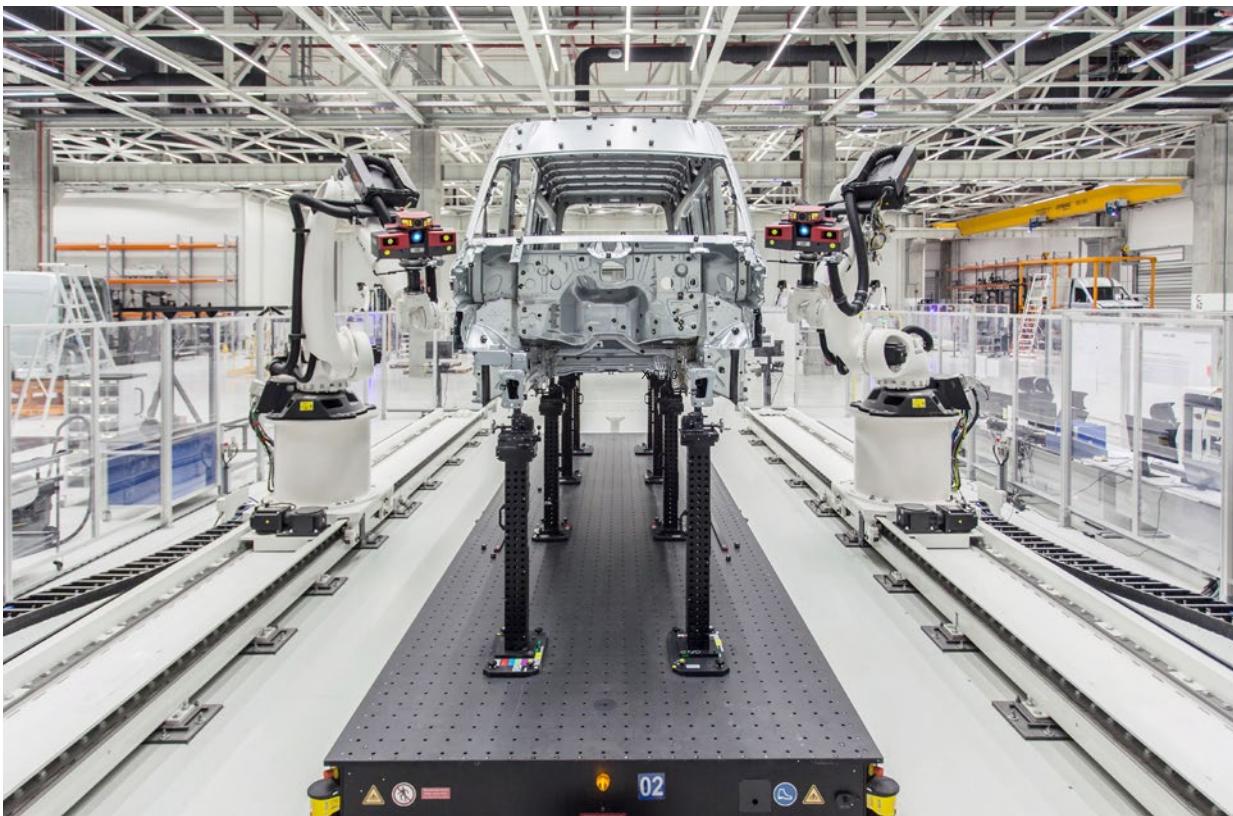
Fig. 2: Inspection of VW Crafter BIW in a double robot measuring cell
