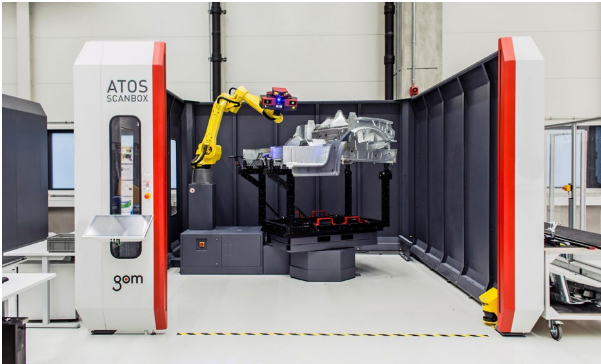
Fig. 4: Underbody part inspection in ATOS ScanBox Series 6
