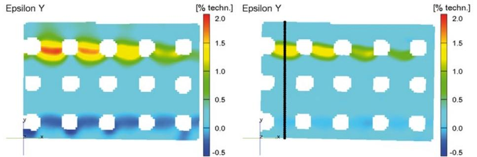
Fig. 8: Graphical display of the epsilon strain values in vertical direction, in the left image at load stage 80 before failure and in the right image, at load stage 84, after failure
