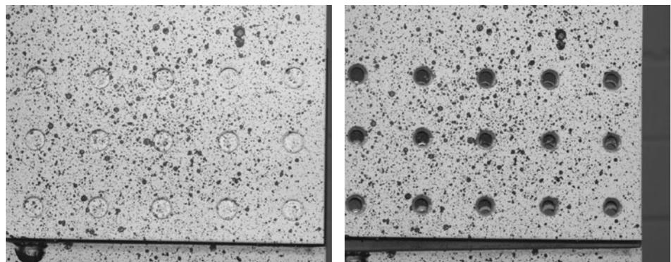
Fig. 7: Sample, at load stage 80, in the left image. In the right image, the sample after failure is visible, at load stage 84
