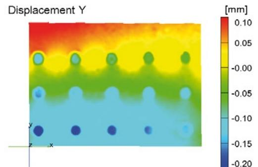
Fig. 4: Relative displacement in tensile direction (Y-displacement), load stage 60
