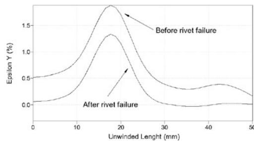
Fig. 9: Plot of the section, shortly before and after the complete failure
