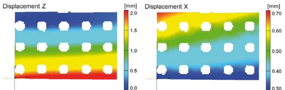
Fig. 5: Deformation values of the load stage 60, referenced to load stage 0. Visible in the left image is the Z-movement (in viewing direction) and in the right image the vertical displacement, in X direction
