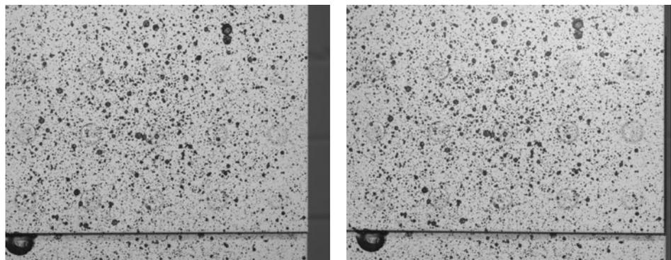
Fig. 1: Sample with splash pattern. The two images show the overlapping area of the two sheets, with the rivets in three rows, before load was applied
