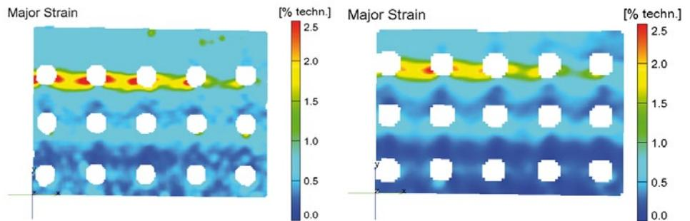
Fig. 6: These images show the major strain at load stage 80, calculated for the left image using a base length of 0.57 mm and for the right image with a base length of 1 mm
