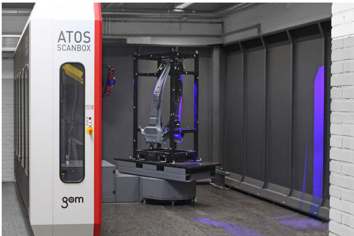
Fig. 1 The ATOS Triple Scan sensor – core of the ATOS ScanBox at Metalsa – allows precise measurements of reflecting sheet metal parts and sharp-edged features such as laser trimming and hole patterns.
