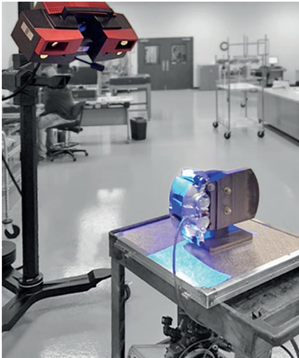
At TRW, components are measured with the 3D scanner ATOS. The illustration shows a brake caliper, which is loaded with 100 bar. To analyze the deformation, the scan data are compared with CAD or an unloaded component.
