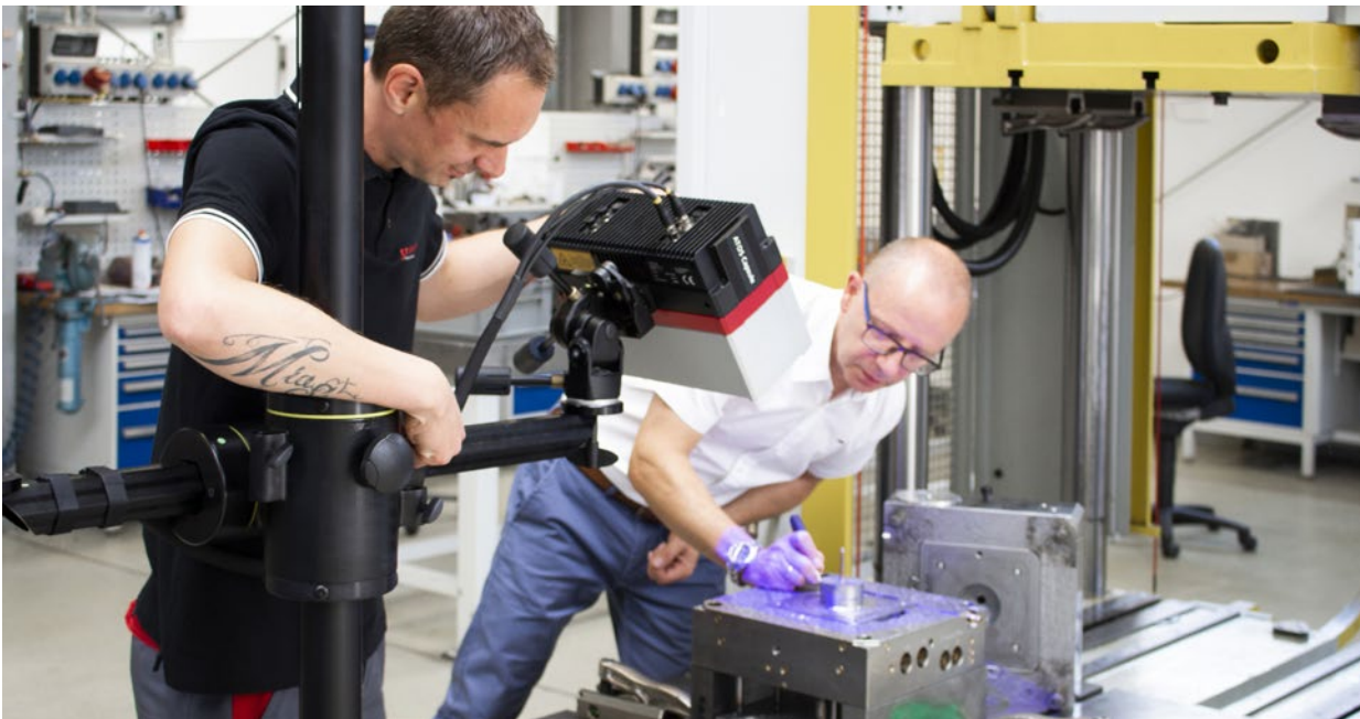
Fig. 1: The ATOS Capsule is used directly during production to check the tool inserts. In the image: Managing Director Ulrich Seifferth and employee Maik Muschko
