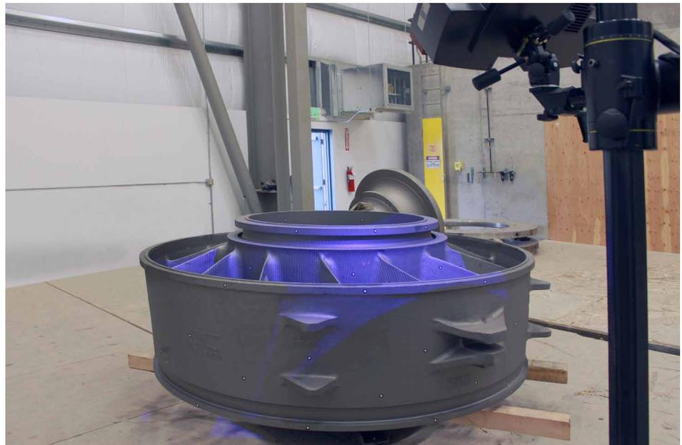
Fig. 3: Blue Light Technology, the narrow-band blue light of the projection unit, allows measurements to be taken independent of ambient lighting conditions and better scanning of shiny surfaces.
