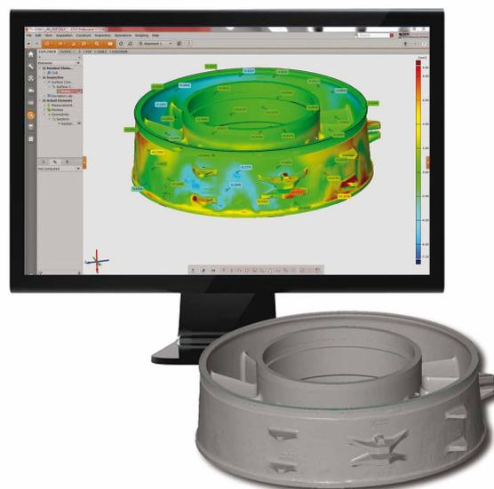
Fig. 2: Tests conducted in Tacoma demonstrated that, within eight hours, ATOS Triple Scan, an optical 3D fringe projection scanner, was able to deliver precise scans with the specified tolerances along with an extensive analysis of the complete casting.
