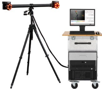
Fig. 1: PONTOS system for optical dynamic 3D analysis, sensor, tripod, computer, (typical measurement set-up)
