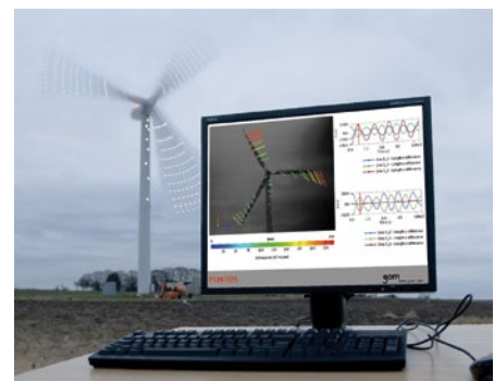
Fig. 4: Online deformation measurement of a wind power plant. The PONTOS system enables analysis of vibrations, frequencies, torsion, bending, speed, acceleration and trajectories
