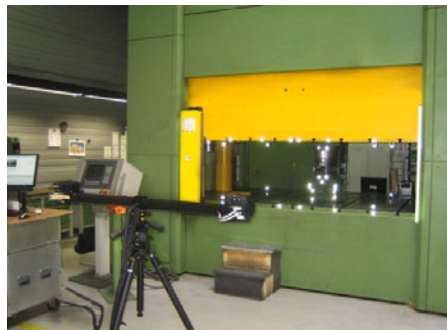
Fig. 8: PONTOS measurement set-up in the production environment.
