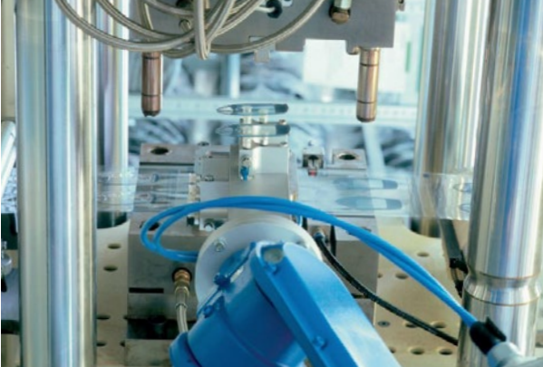
By using the GOM measuring system, the number of correction loops during tool production was reduced from seven to three (Image: Oechsler)
