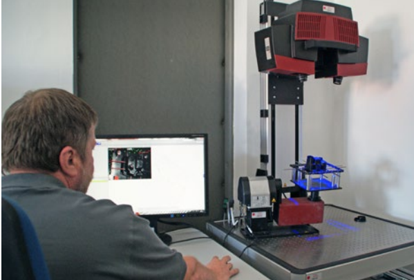
The 3D digitizer enables simple, fast, and reliable measurement workflows at Oechsler (Image: GOM)
