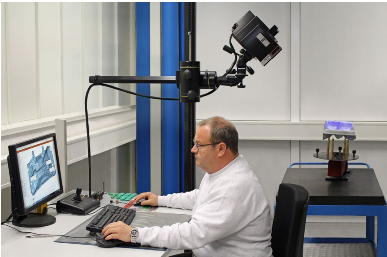
Fig. 2: Wilfried Braun, measurement engineer at PWO, checking the tolerance of a motor mount
