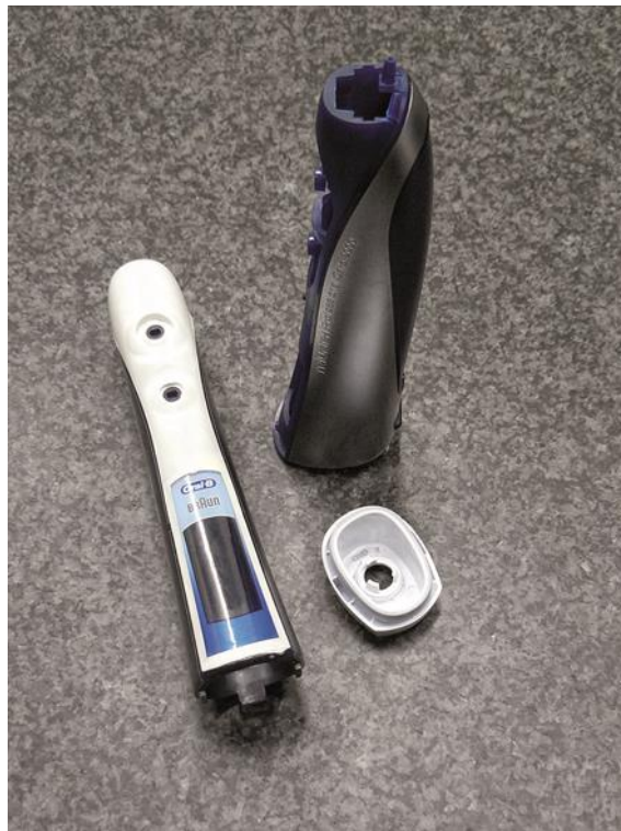
Fig. 3: Especially these housings change their geometric properties after mechanical tensioning and galvanizing. Since tactile methods only sample individual points, these parts used to be very difficult to measure and evaluate. Furthermore, it was almost impossible to measure the 3D seals that Braun integrates in these parts using tactile measurements.
