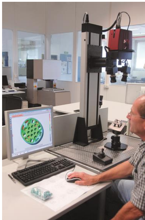
Fig. 1: The ATOS 3D digitizer captures the entire surface of the part instead of just a few individual points. For a complete evaluation Braun uses the GOM inspection software. With its parametric kernel, the software executes inspection processes automatically for components of identical design.
