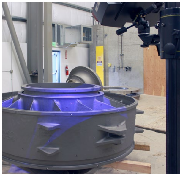
Fig. 3: Blue Light Technology, the narrow-band blue light of the projection unit, allows measurements to be taken independent of ambient lighting conditions and better scanning of shiny surfaces.
