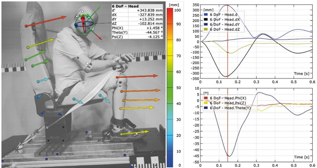
Figure 2: ARAMIS combines point-based and full-field deformation measurements within one measurement system and shows 3D displacement vectors (left) and a full 6DoF analysis (right) of the rotatory and translatory movements of the dummy's head. Trajectories of the head can also be evaluated.
