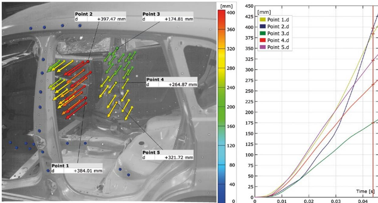
Figure 1: During a side impact crash test, ARAMIS shows 3D displacement vectors while additionally measuring real speed and acceleration. The results can be visualised in easy to understand reports.
