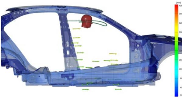
Figure 3: Based on the measuring data, test engineers can analyze precisely how the dummy's head and body will move inside the car. This in turn makes it possible to draw conclusions about the safety of seat and belt systems, but also shows whether there is a risk of head impact inside the vehicle.
