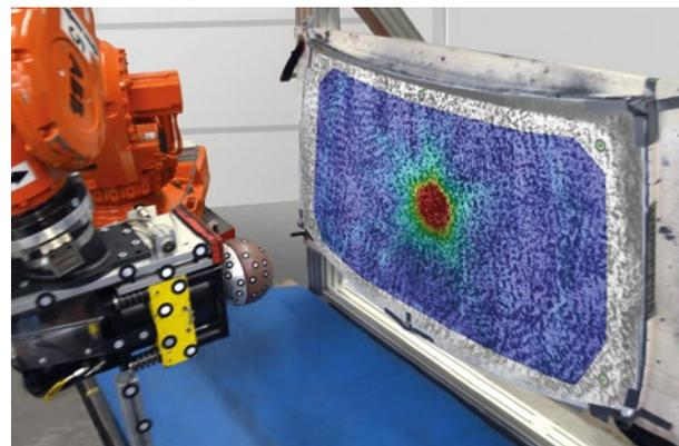
Figure 4: The full-field measuring data recorded by the ARAMIS system can be used to draw reliable conclusions on crack propagation in a windshield.
