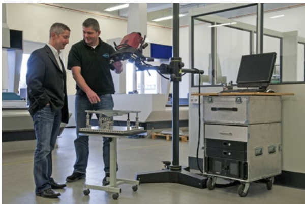
Fig. 2: GEDIA launched the transition from tactile to optical metrology by investing in a mobile ATOS 3D scanner for full-surface optical 3D coordinate measurement. The measuring data can be analyzed immediately and compared directly with the CAD data. Deviations to CAD are highlighted in color and problematic areas are easy to recognize, enabling specific improvements to be made to the manufacturing process.
