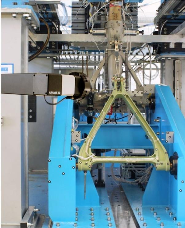
Fig. 3: The optical system can be easily integrated into the test setup, with inspection points identified by measurement markers.
