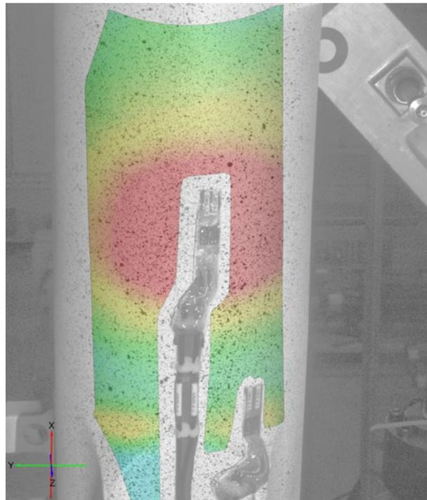
Fig. 2: Full-Field displacement and strain measurement.
