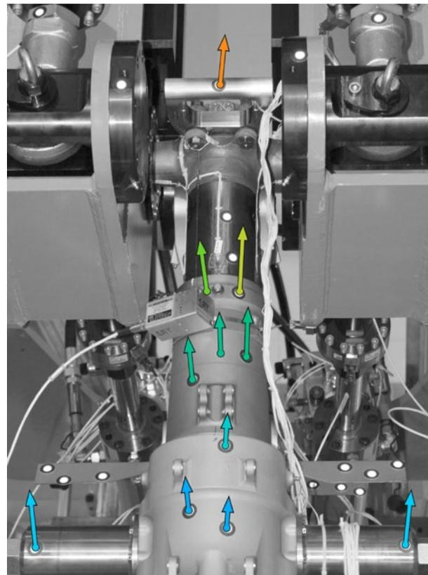
Fig. 1: ARAMIS delivers measuring data for part geometries as well as three-dimensional displacements and provides information about the behavior of the components under load.
