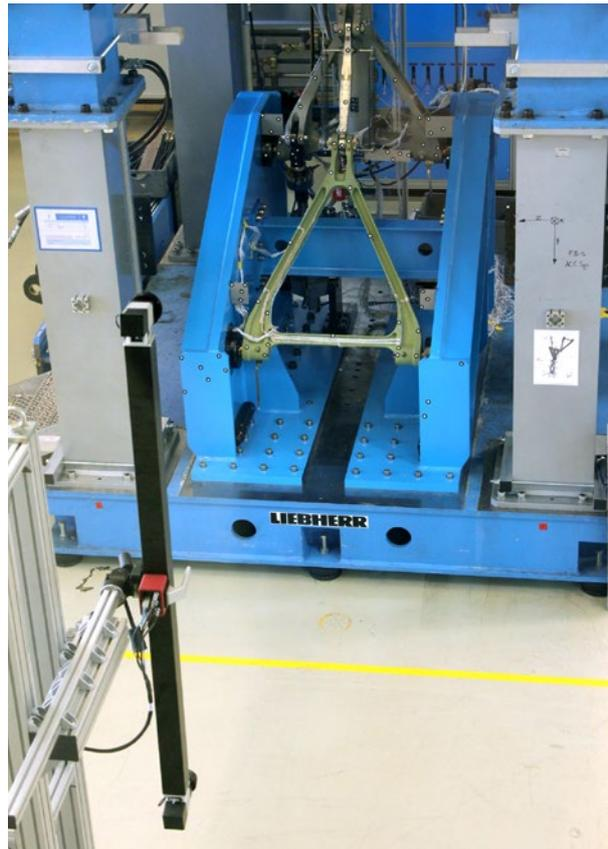
Fig. 4: The new landing gear – placed within an individually designed test rig at Liebherr Aerospace's testing facility in Lindenberg.
