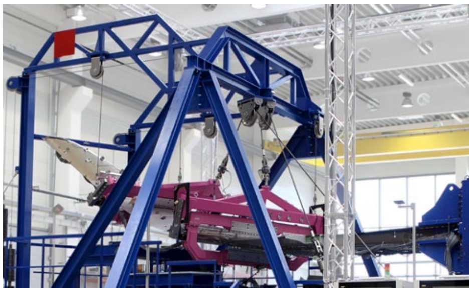
Fig. 1: The winglet is 8m long, 2m high and 3m wide. Around 110 tons of steel were used on the test stand. For the first time, FACC fully integrated non-contact sensors from GOM in the test setup.
