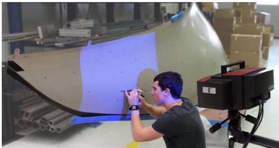
Fig. 4: For an accelerated test setup, the ATOS 3D scanner performed a back projection of the strain gauge positions.
