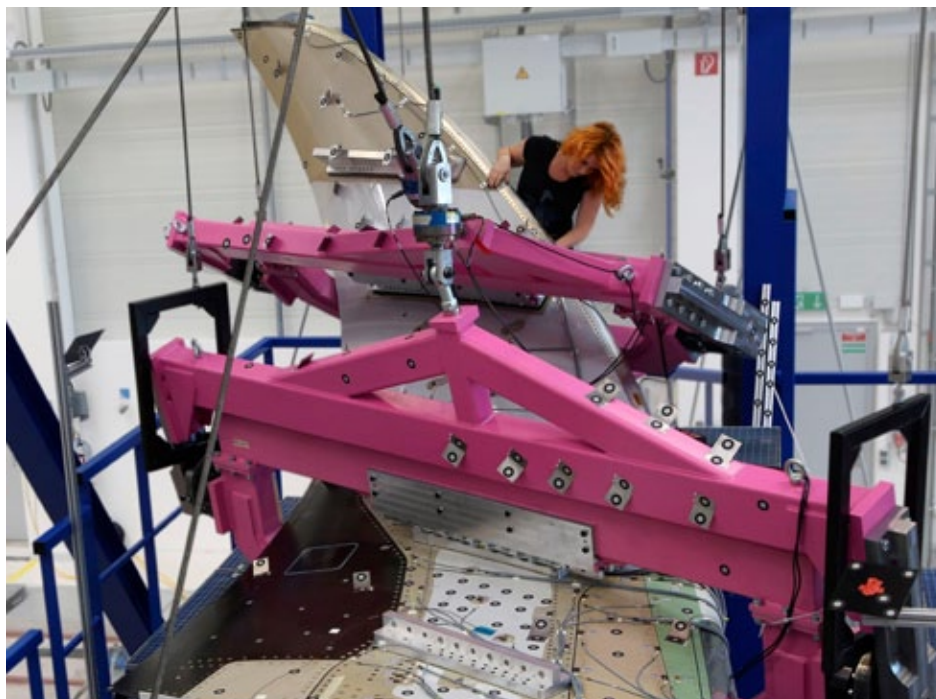
Fig. 2: The PONTOS sensors measure the dynamic deformations at around 220 points, each of which can be analyzed three-dimensionally.
