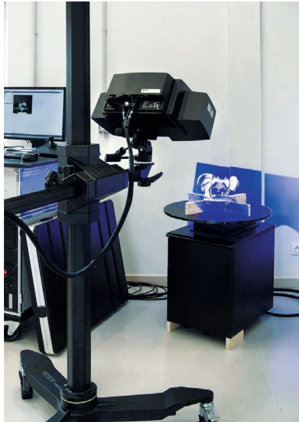
Semi-automatic measurement: GOM ROT 640 (Image: MOB)
