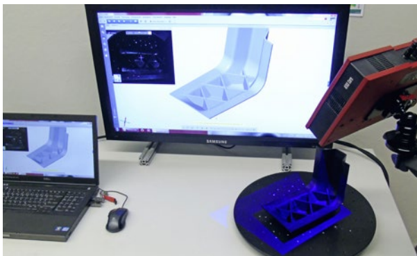
Fig. 5: Nominal vs. actual: The optical ATOS 3D scanner digitizes the "Chemnitz hook" demo component, consisting of a U-profile with rib structure. The software represents the deviations in false color, among other things. (© TU Chemnitz)
