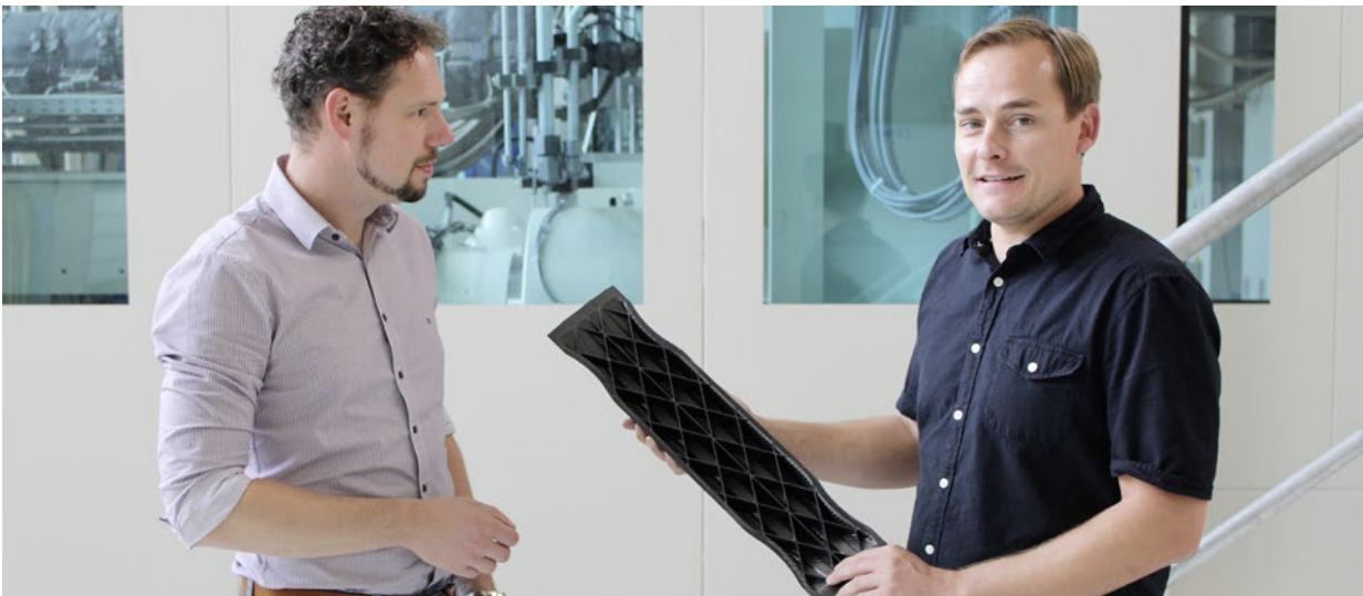
Fig. 2: Norbert Schramm (right) presents a lightweight side impact beam developed by the MERGE team. The injected rib structure increases stiffness (© GOM GmbH)
