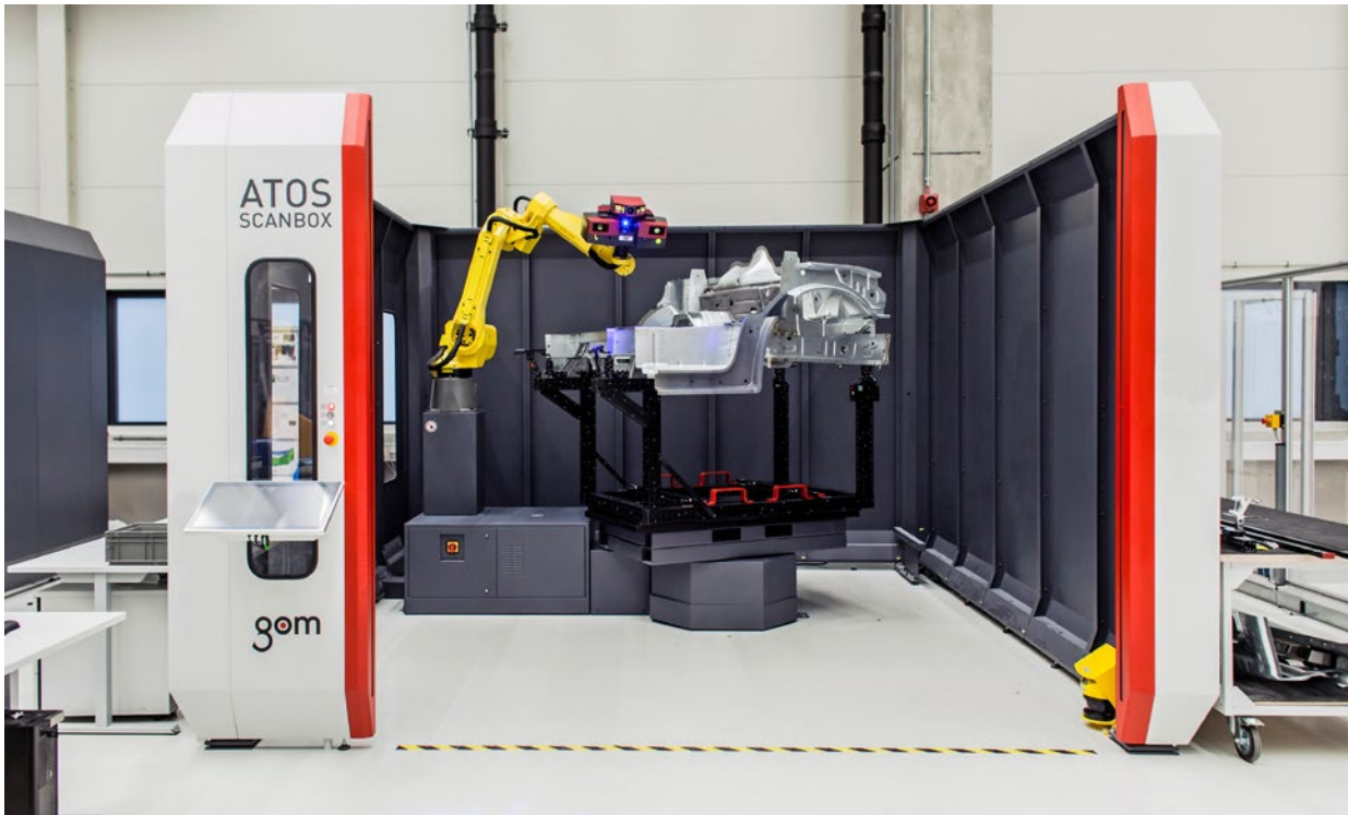
Fig. 4: Undeboddy part inspection in ATOS ScanBox Series 6
