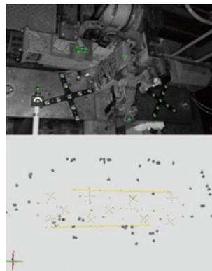
Fig. 4b: Measuring images and 3D coordinates of the reference points
