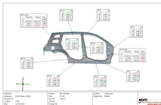
Fig. 6: Measured contact points and their deviation from the nominal position, displayed with CAD data.
