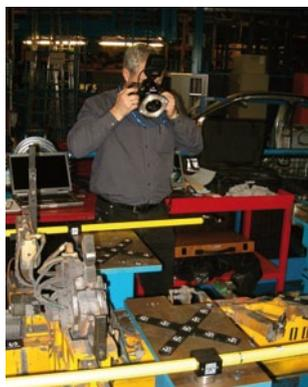
Fig. 4a: Measuring using the TRITOP camera
