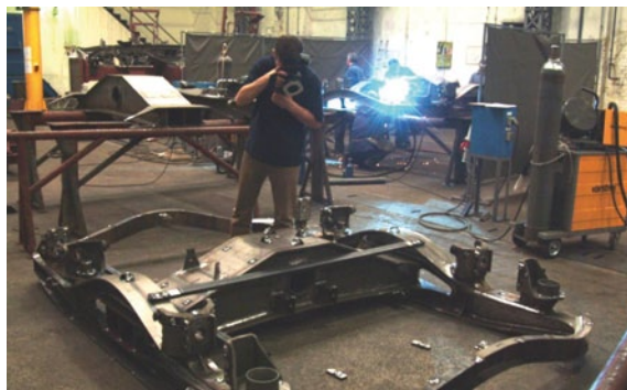
Fig. 5: Taking photos to measure the connection areas and important dimensions of the swivel-truck.
