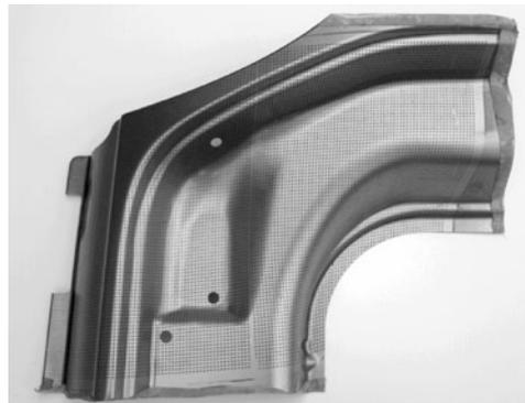
Fig. 1: Stamped part with point pattern
