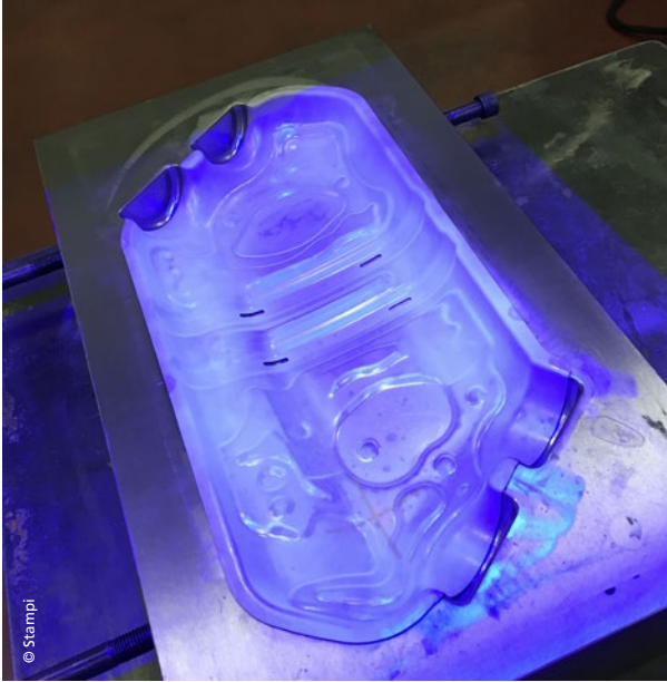
Measurement of a forming tool with ATOS (Blue Light Technology)
