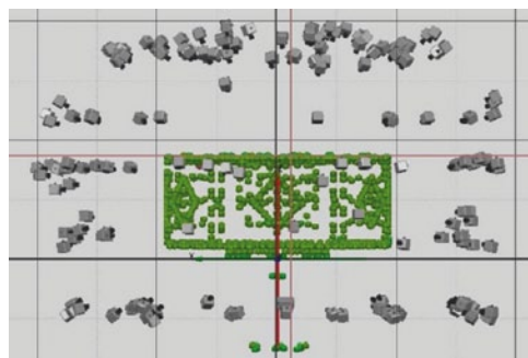
Fig 4: Overview of the camera positions used to generate the images of the test article
