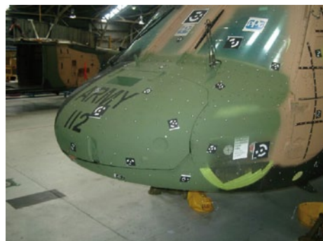
Fig. 5: Nose - prepared for scanning with ATOS
