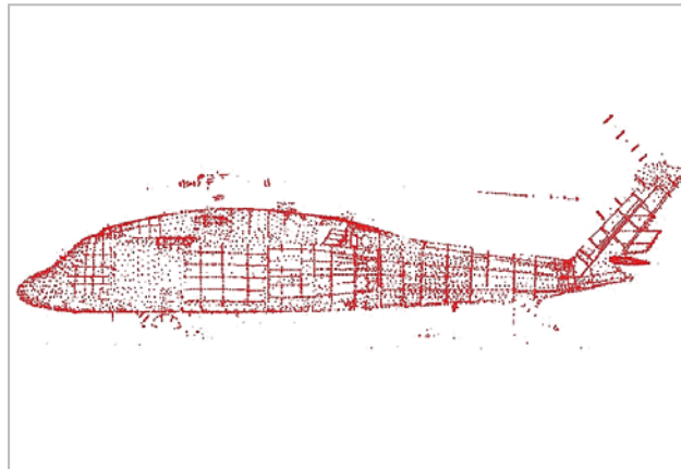
Fig. 4: External skin panels - Scan data established by TRITOP (photogrammetry) (9,000 points, accuracy of 0.1 mm, object size > 15 m)
