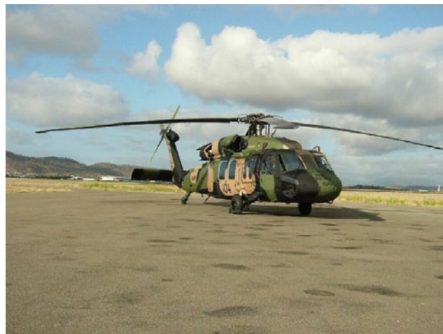
Fig. 1: Black Hawk Helicopter from the Australian Army, Fuselage Size: 15.4 x 2.4 x 2.3 meters (Length, width and height)
