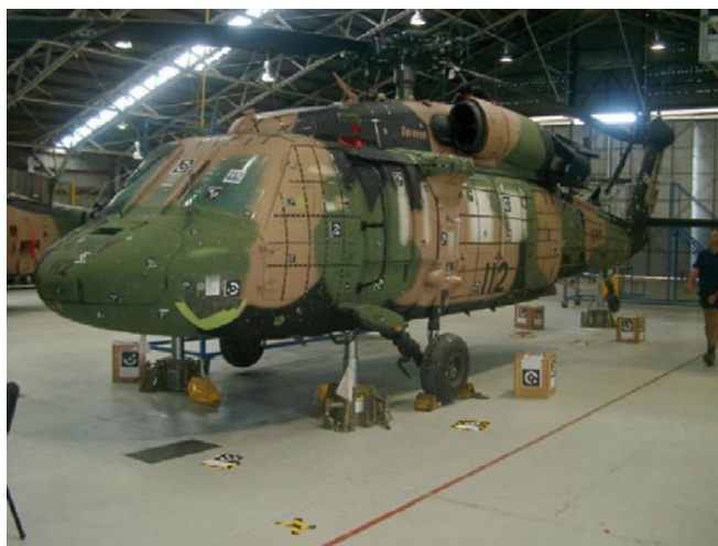
Fig. 3: Fuselage prepared for scanning
