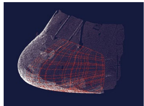
Fig. 6: Nose - ATOS Scan data (optical white light scanner data)
