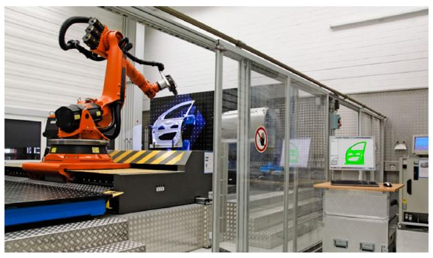
The robot measurement cell allows unmanned and time-saving inspection of sheet metal components ranging from lock plates to complete side panels.
