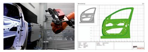
Fig. 2: The fringe projection process and stereo camera principle in optical metrology guarantee accurate and reliable component inspection. Full surface measurements enable complete component inspection and a clear view of results, thus saving time on component evaluation.
