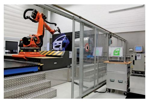
Fig. 1: The robot inspection cell enables BMW to save time inspecting sheet metal components ranging from lock plates to complete side panels without the need for operator intervention.
