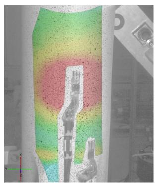
Fig. 2: Full-Field displacement and strain measurement.
