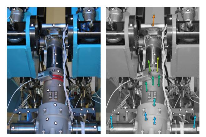
Fig. 1: ARAMIS delivers measuring data for part geometries as well as three-dimensional displacements and provides information about the behavior of the components under load.
