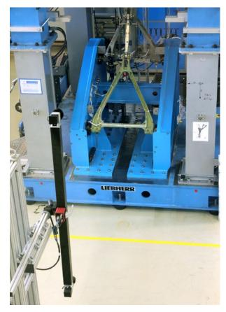
Fig. 4: The new landing gear – placed within an individually designed test rig at Liebherr Areospace's testing facility in Lindenberg.
