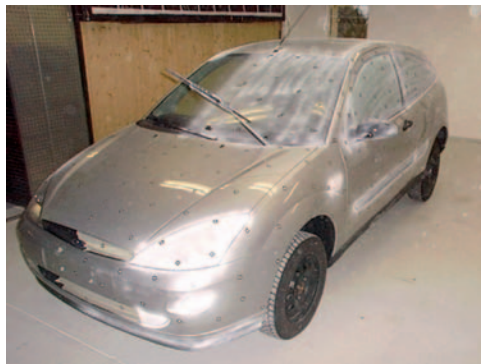
Fig.1: Digitizing of a Ford Focus
