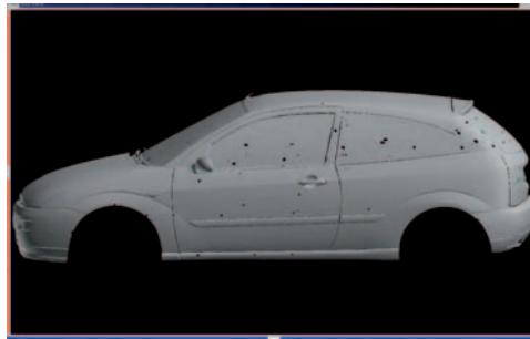
Fig.2: Individual digitized areas are matched together for complete data set
