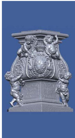
Fig. 5: Flat shaded view of the scanner data as given by ATOS of the statue.
